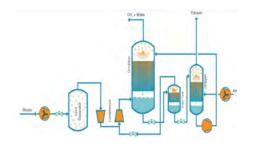
Compressed Bio Gas Compressor Suction: 5 ~ 7 barg Discharge: 250 barg Flow: 300 to 400 SCMH
