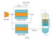
Compressed Bio Gas Compressor Suction: 9 ~14 barg Discharge: 250 barg Flow: 400 to 1200 SCMH
